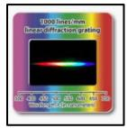
A device used to break light into its component wavelengths. It is usually composed of a material with tiny grooves cut into it. These disperse the light as it passes through or bounces off the grating (depending on the type of grating).
