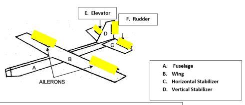
**Right Bank:** Right aileron is up; left aileron is down
