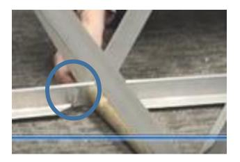
HINT: Use the big screws for the supports and side trusses. Use the little screw for the top bar.
