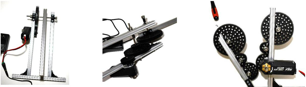
**Manipulator B:** Student has supplies to build manipulators that involve servos. They use the programmable servo to power and test the servos in their manipulator.
